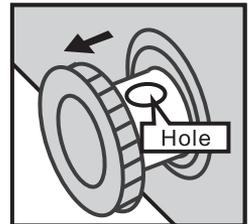
**Note:** Monitor the tray under the drain, emptying as required to avoid water overflowing
