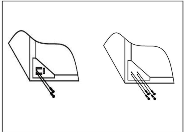
3. Remove the casters from the bag and insert them into the slot at the bottom corner of the refrigerator or onto the mounting holes.
