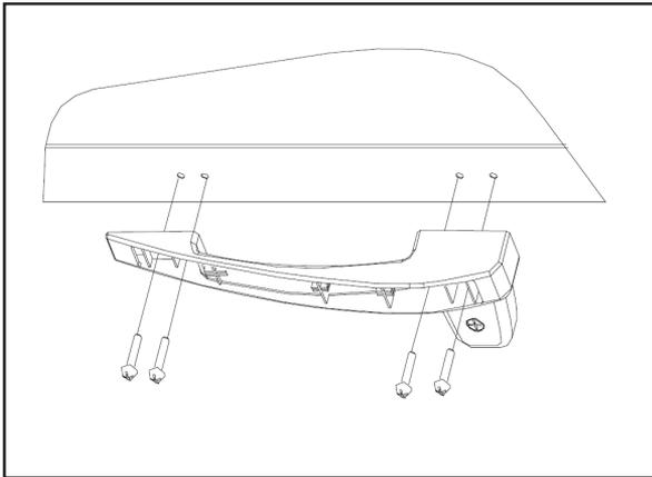
2. Insert the one side of handle cover into the handle pedestal.
