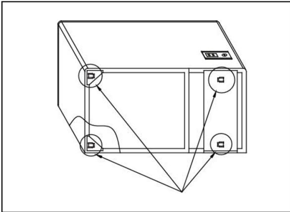
2. Remove the screws at the bottom four corners of the chest freezer.
