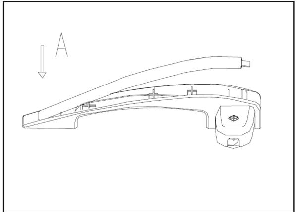
3. Insert the other side of handle cover into the handle pedestal.
