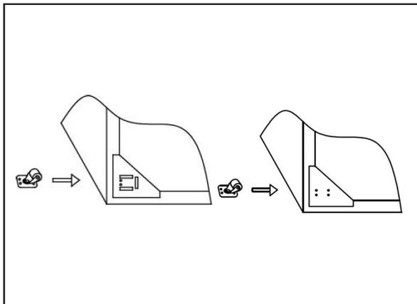
4. Align the holes on the casters with the holes in the case, install and tighten the screws.
